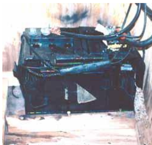
Visible are the exploded plastic case exposing some of the internal plates as well as battery acid damage to the nearby wood walls and flooring.
