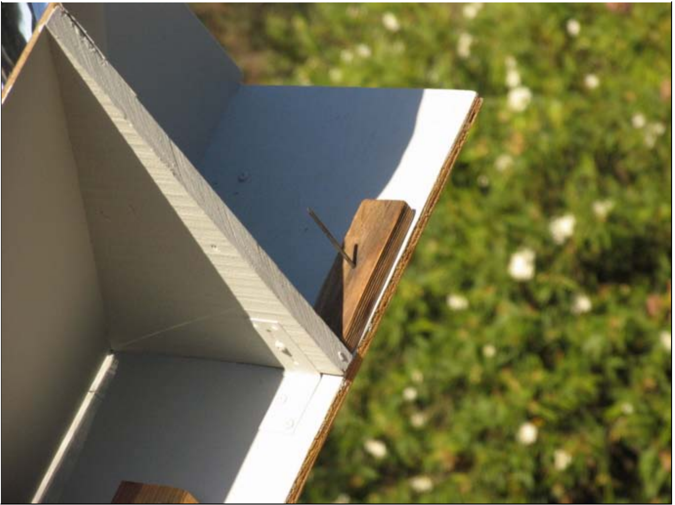
The gnomon shows that the oven is "ahead" of the sun, meaning that the sun will need to rise further, and travel a bit further west so as to be normal to the collector plate. I generally keep the oven ahead of the sun.
