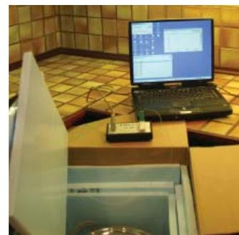
**Figure 2 - RHC made with a cardboard box**
