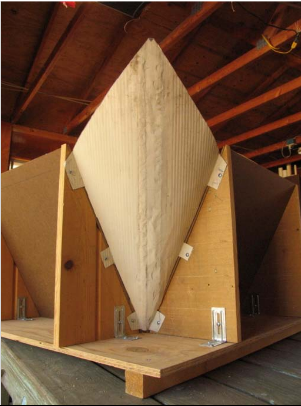
The reflective film has been glued to the front surface, and the insert is now attached to the supports. Here I use 8-18 x 1/2" self-drilling screws, but I always drill pilot holes nonetheless.
