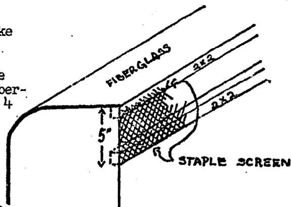
**12: SCREENING VENT OUTLET:** Staple 6" x 48" of screen along the edge to a 46½" long 1 x 2, nail the screen, facing back. (See Figure 10.) Staple the screen to the 2 x 2 and the 1 x 10's.
