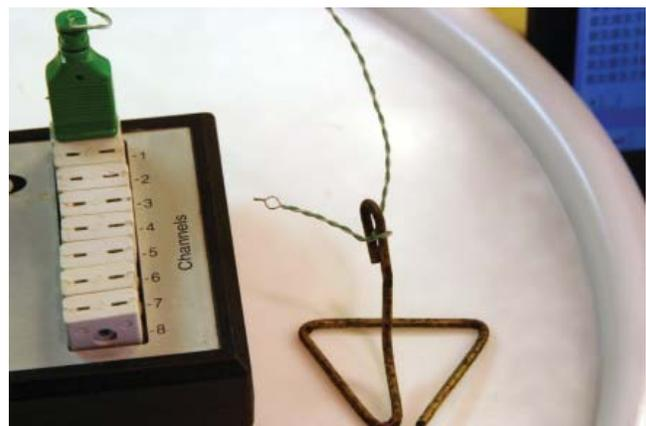
**Photo 1 - Thermocouple Support**
