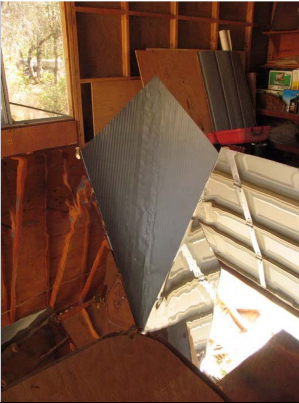
The mock-up from the front. The angle of the insert is acceptably close to the desired 120 degrees off the collector.
