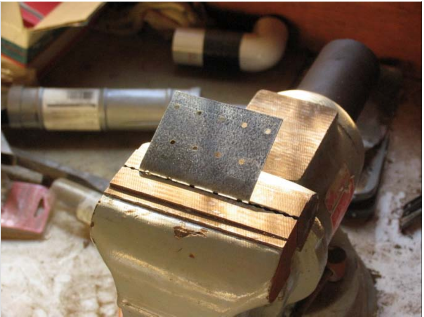
Begin the bend by pushing evenly across the width of the plate. Continue the bend to the top of the vice jaw.
