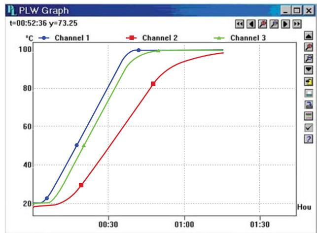
Figure 6 - Internal temperature lag of food in RHC
