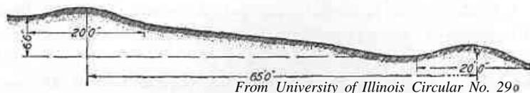
Cross-section of two mangum terraces, 65 feet apart, on a 10 per cent. slope.
