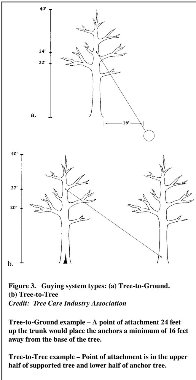
**Figure 3. Guying system types: (a) Tree-to-Ground. (b) Tree-to-Tree**
