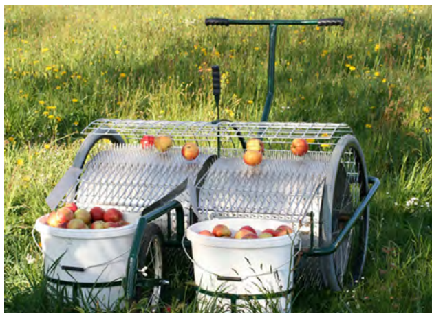
Figure 3.3. Rolling drum harvesters such as these made by Huemer Obsterntechtechnik might be appropriate for smaller cider plantings. Basic models are hand-pushed, with options for adding an electric assist motor. A larger unit can be pushed by a lawn tractor or walk-behind tractor. SOURCE: HTTP://WWW.OBSTSAMMLER.COM/EN/
