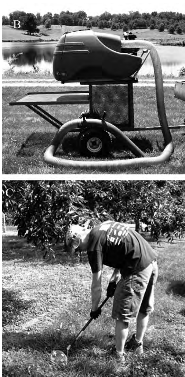
Figure 3.9. Modified pasture vacuum (Maxi Vac, Greystone Vacuums) with raised collection tank and open-weave metal shelf (top) and Nut Wizard (Holt's Nut Wizard, Douglas, GA) (below). PHOTO: WARMUND, ET AL 2013. USED WITH PERMISSION.
