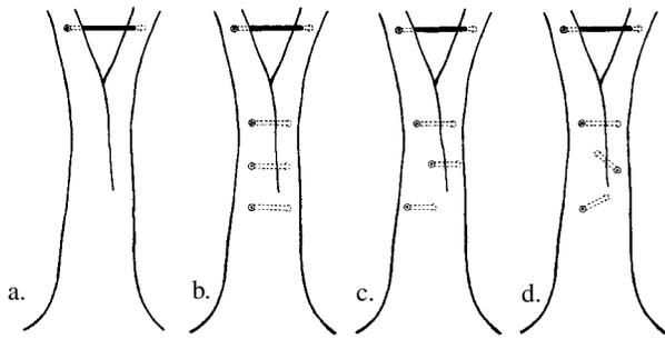
**Figure 1. Bracing system types: (a) Single, (b) Parallel, (c) Alternate, and (d) Crossing**
