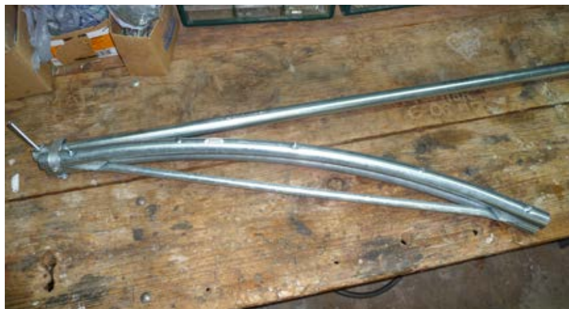
A 'Quick Hoops' tube bender mounted to a shop bench. For more information on this bender, go to http://shop.hoopbenders.net .
