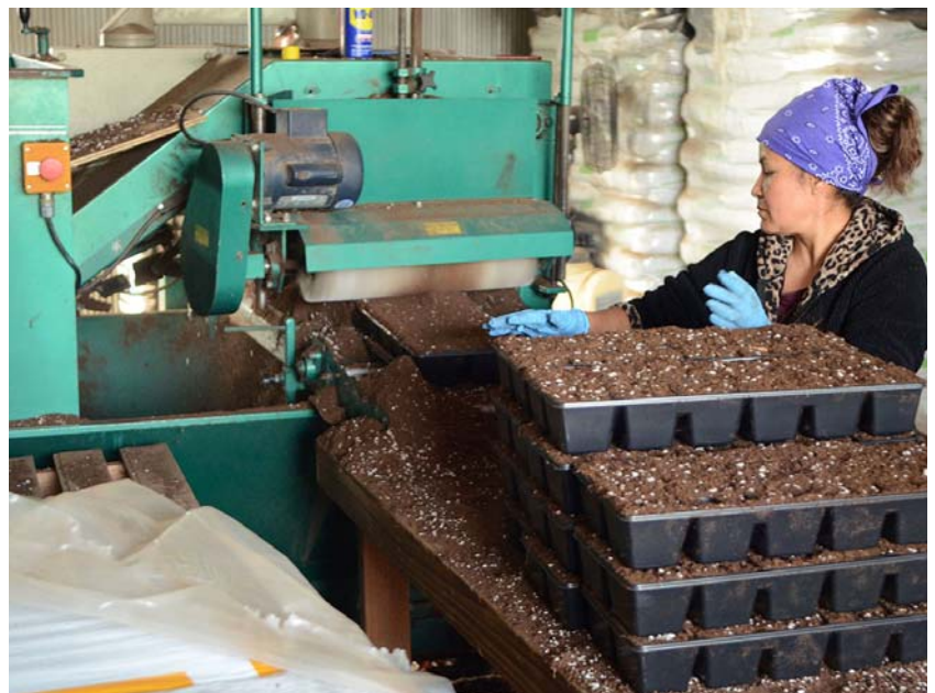
Cell packs are filled with organic media using a mechanized filler at Peace Farm Organics. Photo: Luke Freeman, NCAT
