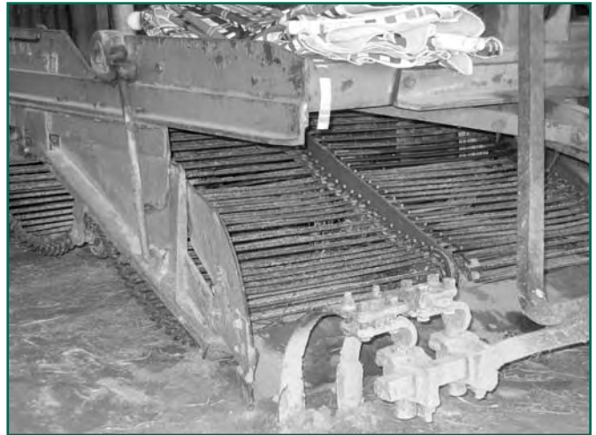
Donovan's two-row harvester cuts under the potatoes and brings the entire hill up and over the moving rods. The dirt falls between the rods and the potatoes are carried to the back and dropped onto the ground. Photo by Jack Kittredge, courtesy of The Natural Farmer.
