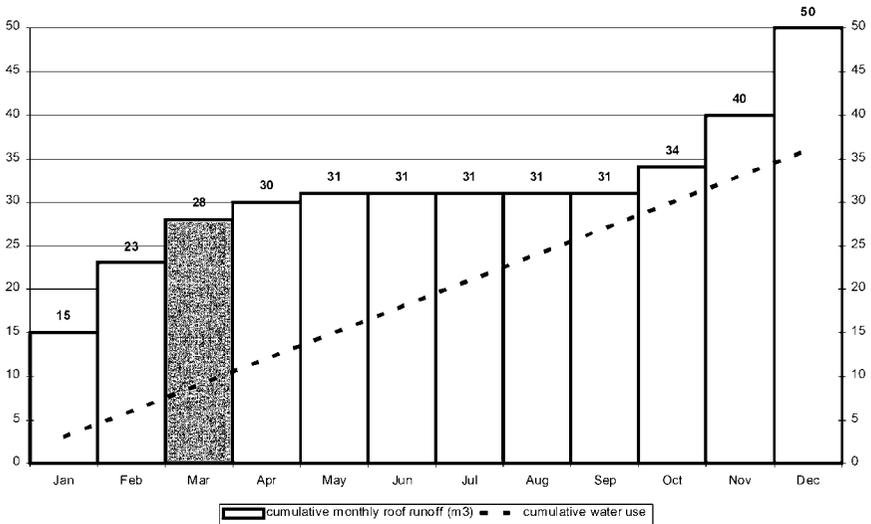
Figure 16: Cumulative monthly roof run-off including a residual storage of 5 m<sup>3</sup> and cumulative water use. Estimation of storage requirement.
