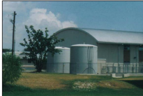
Water collected from the roof of the J.J. Pickle Elementary School and St. John Community Center is stored in three large tanks behind the building and used as cooling water for the complex's air-conditioning system.
