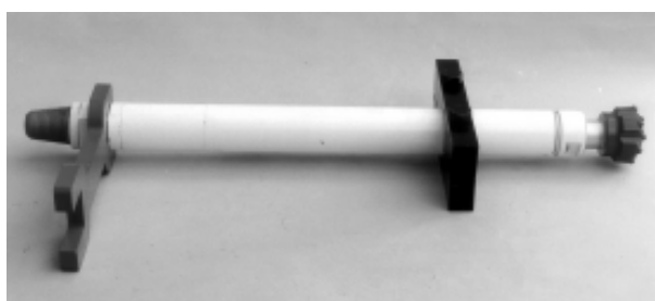
Figure 3.3 Down-the-hole hammer – with stripping clamp and spanner
