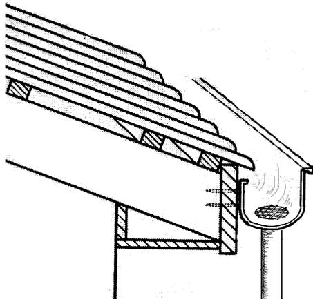
Figure 25: Coarse filter
