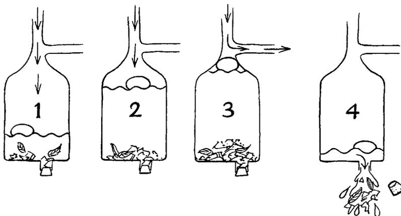
Figure 28: SafeRain system for separating first-flush
