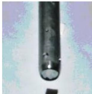
Piston made of rubber and a tool (a punch) to make standardized pistons
