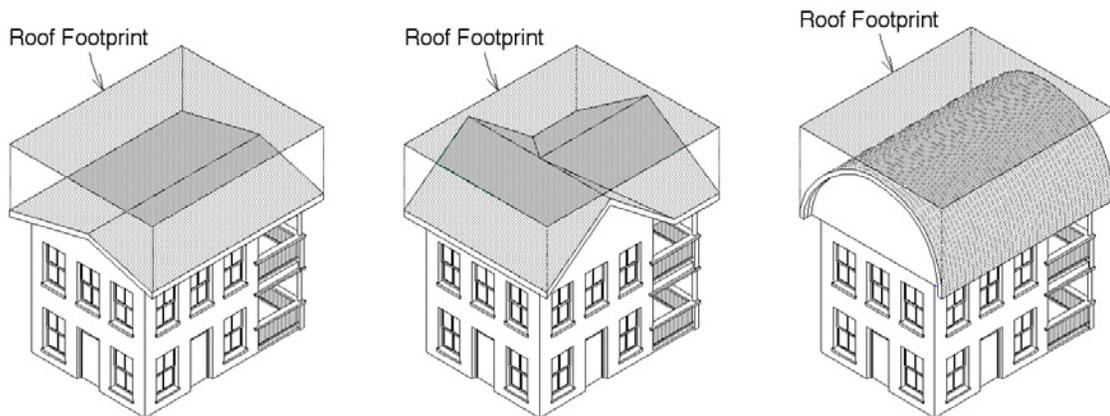
Figure 4-1. Catchment areas of three different roofs
