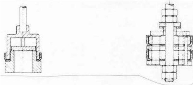
Figure 14 Lay-out of a flat valve design.
