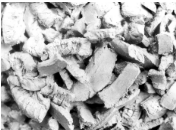
Figure 2.9 Individual clay cuttings washed to the surface
