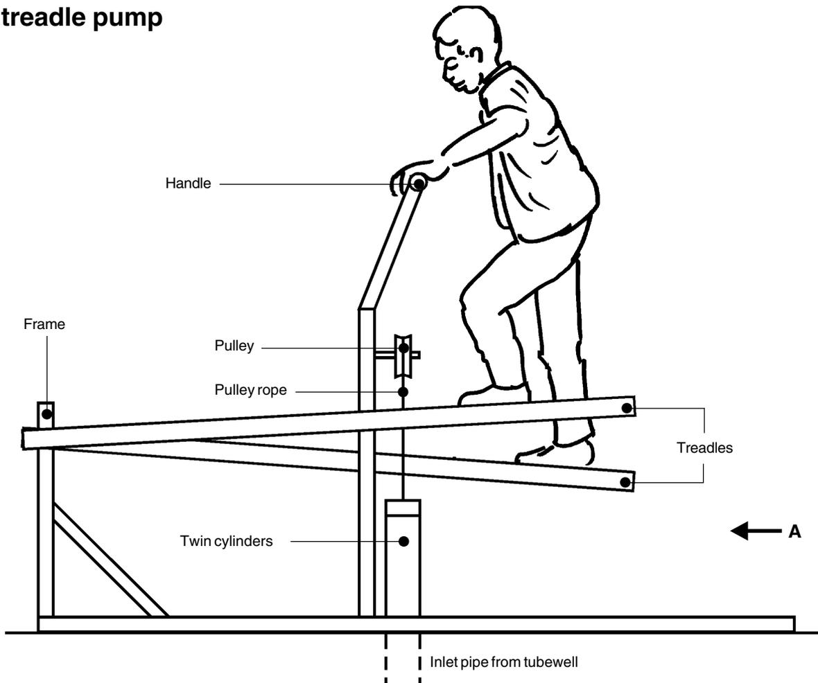
Because the treadle pump is operated by the most powerful muscles of the human body, it can be operated for longer than other human-powered pumps.
