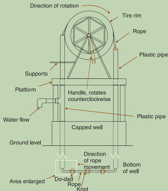
Cross-section of Rope Pump on a handdug well
