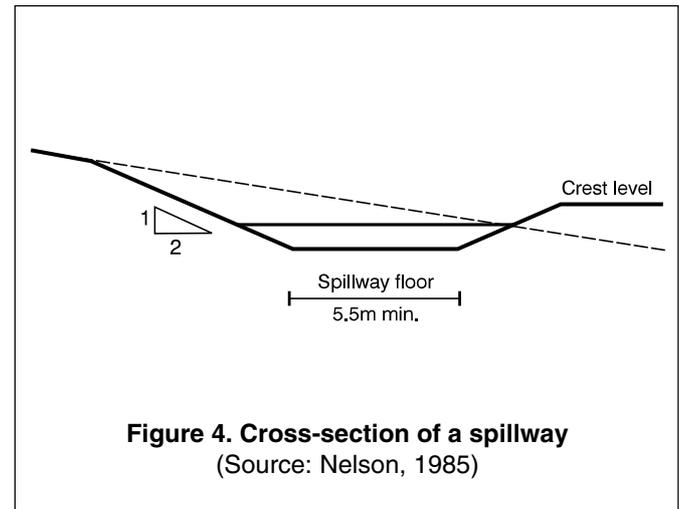
**Figure 4. Cross-section of a spillway**
