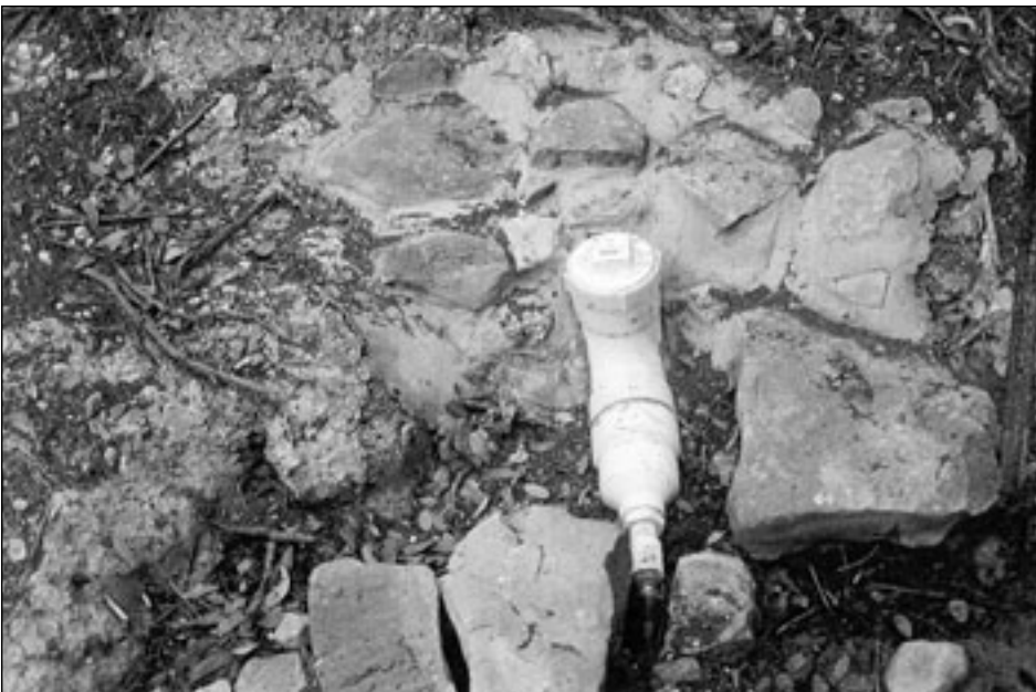
The milking system installed behind the armadillo hole. This is the site Prehn constructed by hand. Site One produces about 500 gallons a day.
