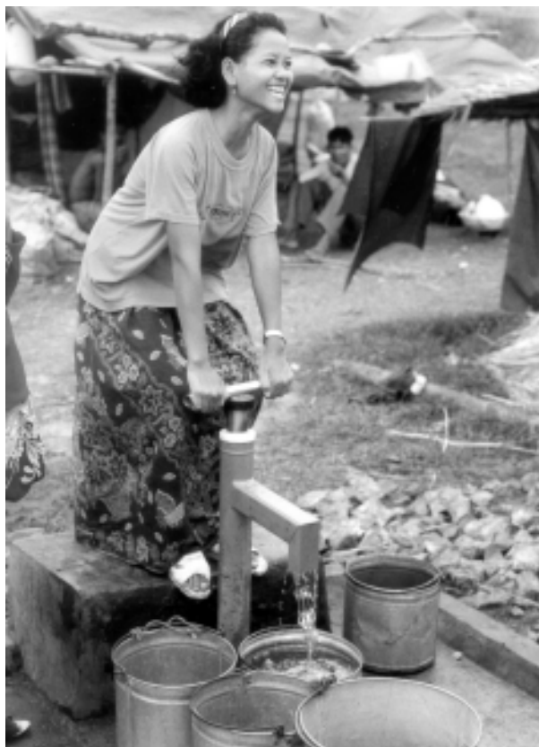
Figure 6.2 Direct Acting hand pump
