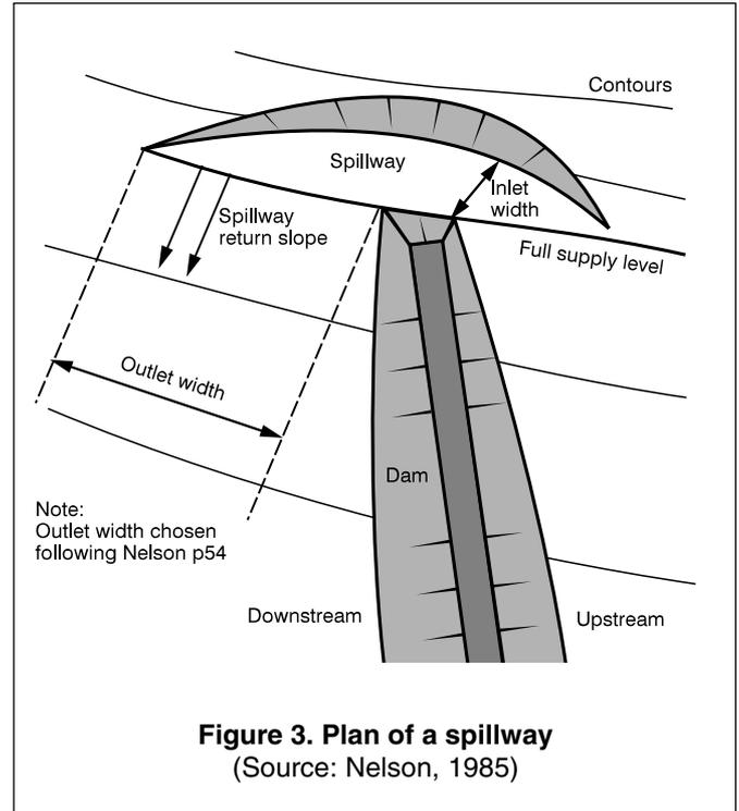
**Figure 3. Plan of a spillway**
